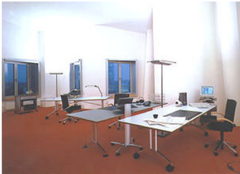
Figure 2: Waveguide-based luminaires produce glare free light for offices utilizing CRT and flat panel displays
