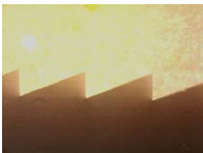
The same view of a fresnel lens molded by Reflexite Display Optics shows sharp facets and greatly improved replication.
